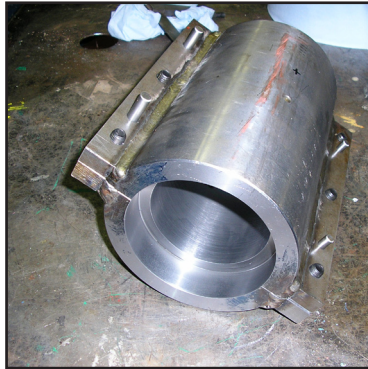
View of former. A stepped former was required to allow it to clamp and locate undamaged areas.
