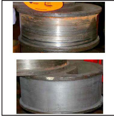
Close up of scored and repaired bottom journal
