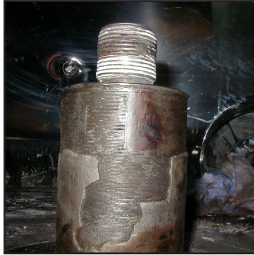
Failed Metal Sprayed Shaft
